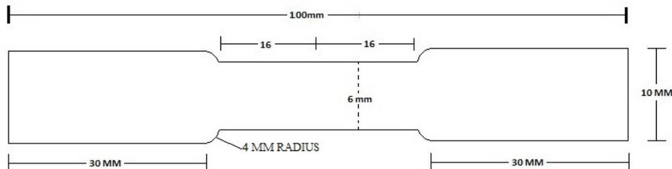
Fig. 1.4: Dimensions of tensile test specimen (in mm)
