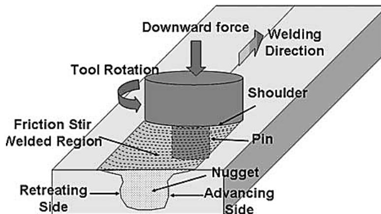
Fig.1.1: Set up of a FSW Process [7].
