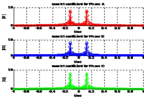
Fig. 6 The coefficient density per phase on the application of wavelet transform
