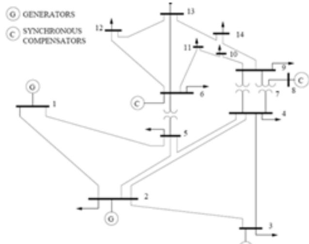
Fig. 3 IEEE-13 Bus system line diagram
