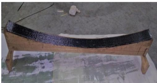
Fig.3 Laying of the cloth on mould
