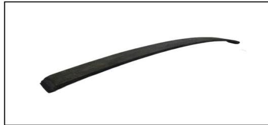
Fig.6 Finished carbon epoxy composite leaf spring
