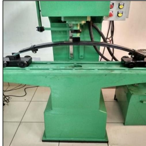
Fig.8 Fatigue testing of steel spring
