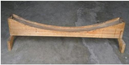
Fig.1 Mould for Composite Leaf Spring
