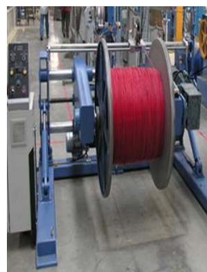
Fig. 4 Pictorial representation of take up machine with PVC layer
