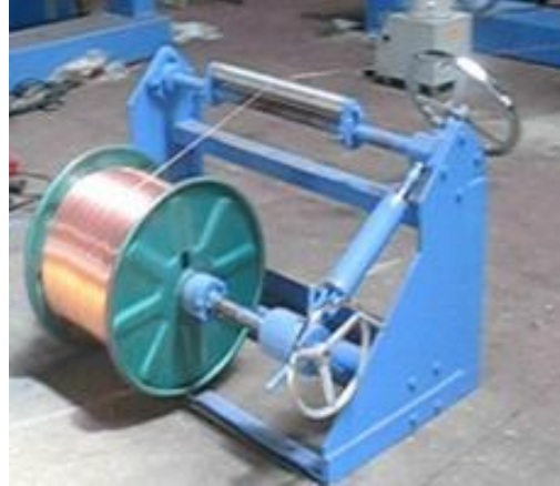
Fig. 7 Cable payoff process
