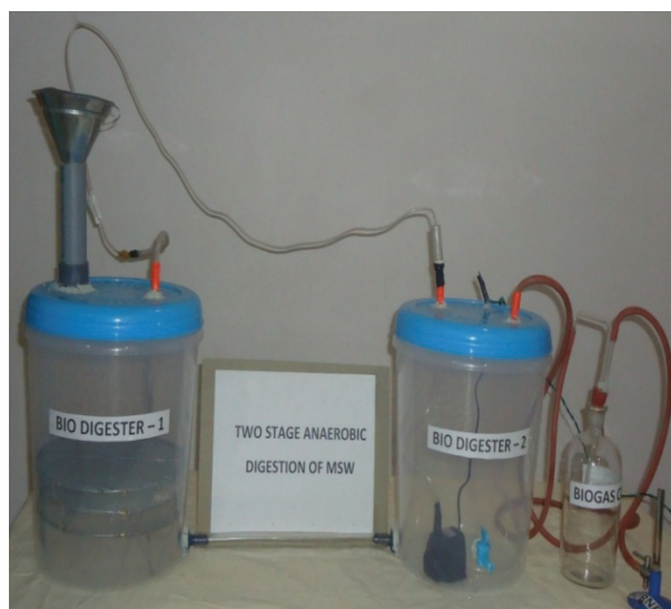
Photo. 2 Working setup of two stage anaerobic digestion system
