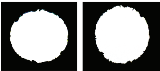
Fig. 1 Microscopic views of micro sinker holes at entry (a) and exit (b) with machining conditions 10V, 100 nF
