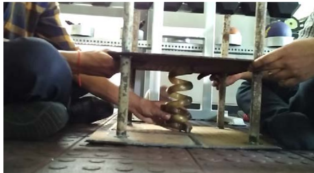
Fig.10 Test rig prepared for deflection testing
