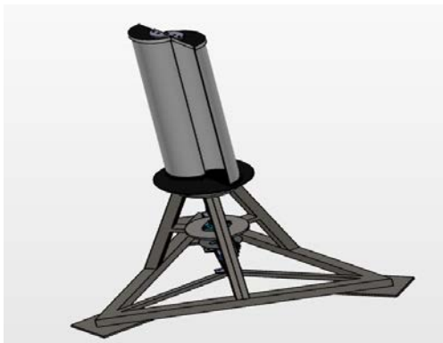
Fig.1 CREO Layout Design of VAWT
