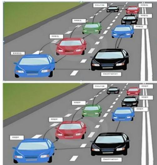
Fig. 7 Routing Propagation in VANET System
