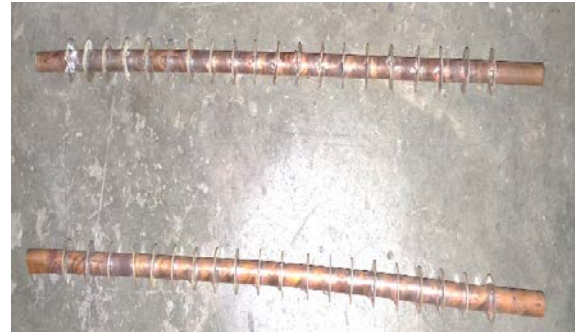
Fig.4 Plain and Perforated Fin Arrays
