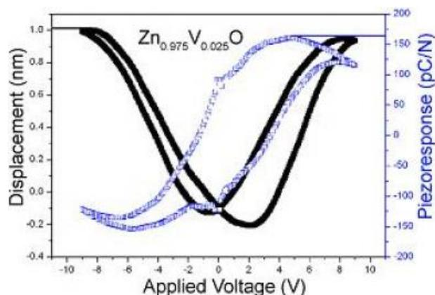
Fig. 3 Representative D-V curve and the piezoresponse hysteresis loop of  $\text{Zn}_{0.975}\text{V}_{0.025}\text{O}$  films[23]
