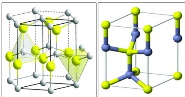
Fig. 4 ZnO structure: (a) the wurtzite structure model (b) the wurtzite unit cell. The O<sup>2-</sup> and Zn<sup>2+</sup> form a tetrahedral unit, and the entire structure lack central symmetry.
